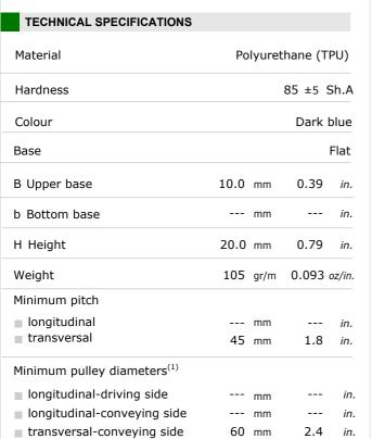
$^{(1)}$  Minimum pulley diameters referred to environment conditions of 20  $^{\circ}\text{C}$
